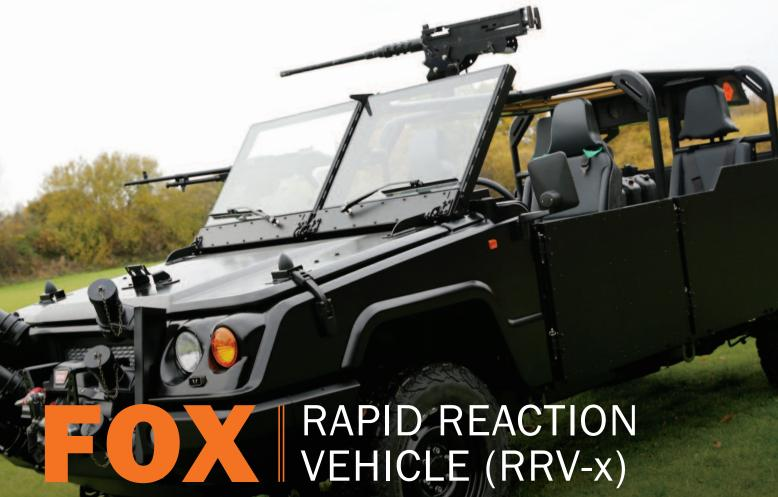
In today's ever changing world, tactical vehicles need the modularity to fulfil a variety of roles in order to offer the most cost effective capability. The Fox Rapid Reaction Vehicle (RRV-x) has been designed with enhanced weight carrying capacity, internal CH-47 air transportability and increased off-road agility to push the boundaries of payload, mobility and performance.
